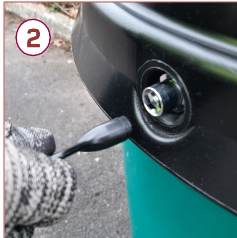
The lock barrel will pop out to show that it is in the unlocked position.
