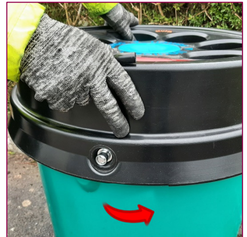
Twist the lid anti-clockwise to disengage the bayonet fitting
