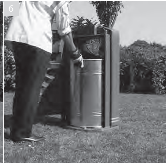
6 Replace liner sliding the liner in until it will go no further
