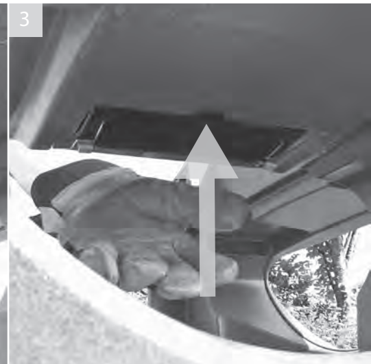
3 Once the contents of the ashtray has fallen into the liner release grip, the sprung hinge will return the flap to its closed position
