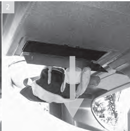
2 Pivot the ashtray flap downwards until it is vertical. Contents will fall into the liner below
